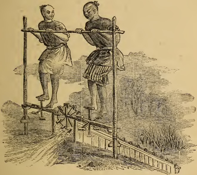
IRRIGATION BY MEANS OF AN ENDLESS CHAIN-PUMP.
