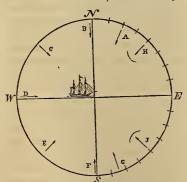
winds represented by the arrows A, B, C, &c., to G. Of these winds, C and E are the best, because they strike all the sails, while a wind from D would not. Pilot boats can go with the wind H and J, i. e. within "four points;" ships cannot go within "six points." Each of the quadrants above are supposed to be divided into eight points, as in the mariner's compass. The wind we have to-day is G, or S. S. E. I'm at a loss to know how you will
